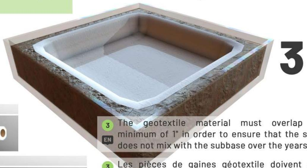
3 The geotextile material must overlap a minimum of 1" in order to ensure that the soil does not mix with the subbase over the years.
